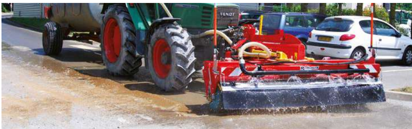
PROCHAMPION on tractor front 3-point linkage
